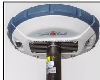
Figure 15- DGPS Survey Instrument
